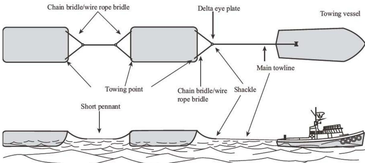
**Figure 1.2 Diagram of tandem tow**
