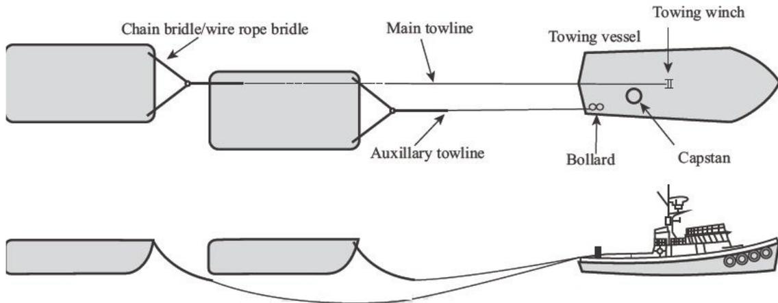
**Figure 1.1 Diagram of double tow**
