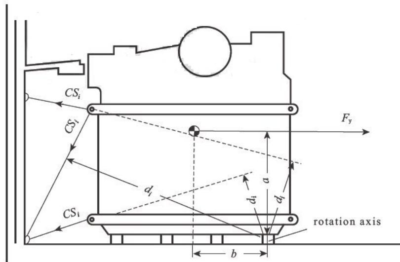
Figure 4.2 Securing forces for transverse tipping
