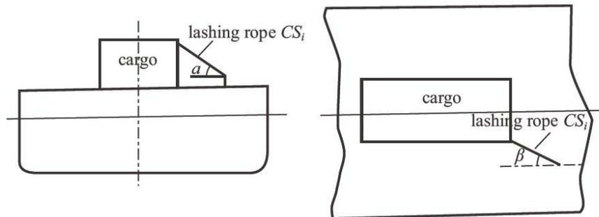
**Figure 4.1 Calculation of angle  $\alpha$  and  $\beta$**
