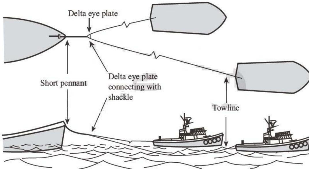
Figure 1.4 Diagram of multiple tugs to one tow
