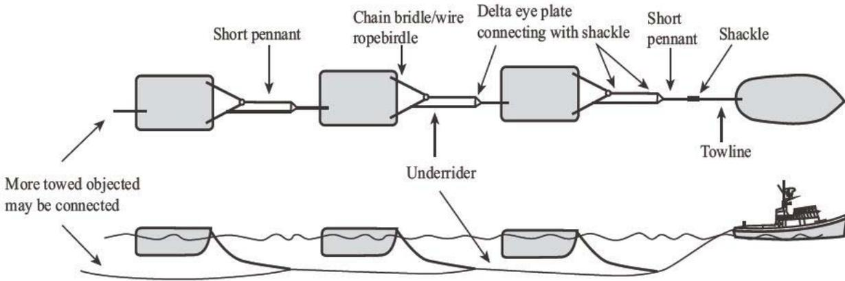
Figure 1.3 Diagram of parallel tow
