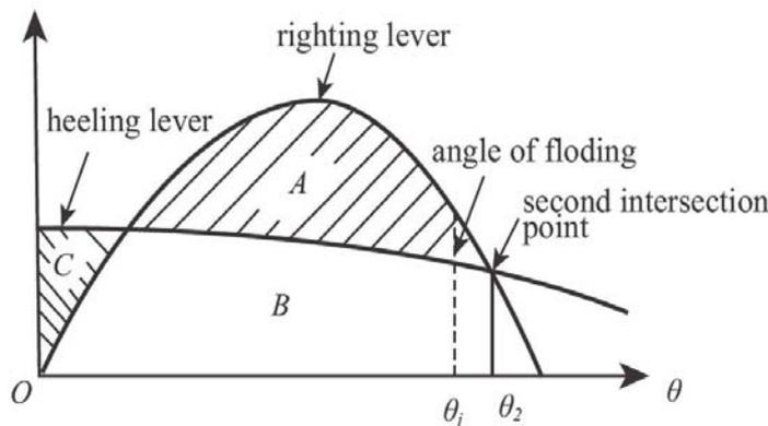
**Figure 3.2.1** Areas covered by righting lever curve and wind heeling curve
